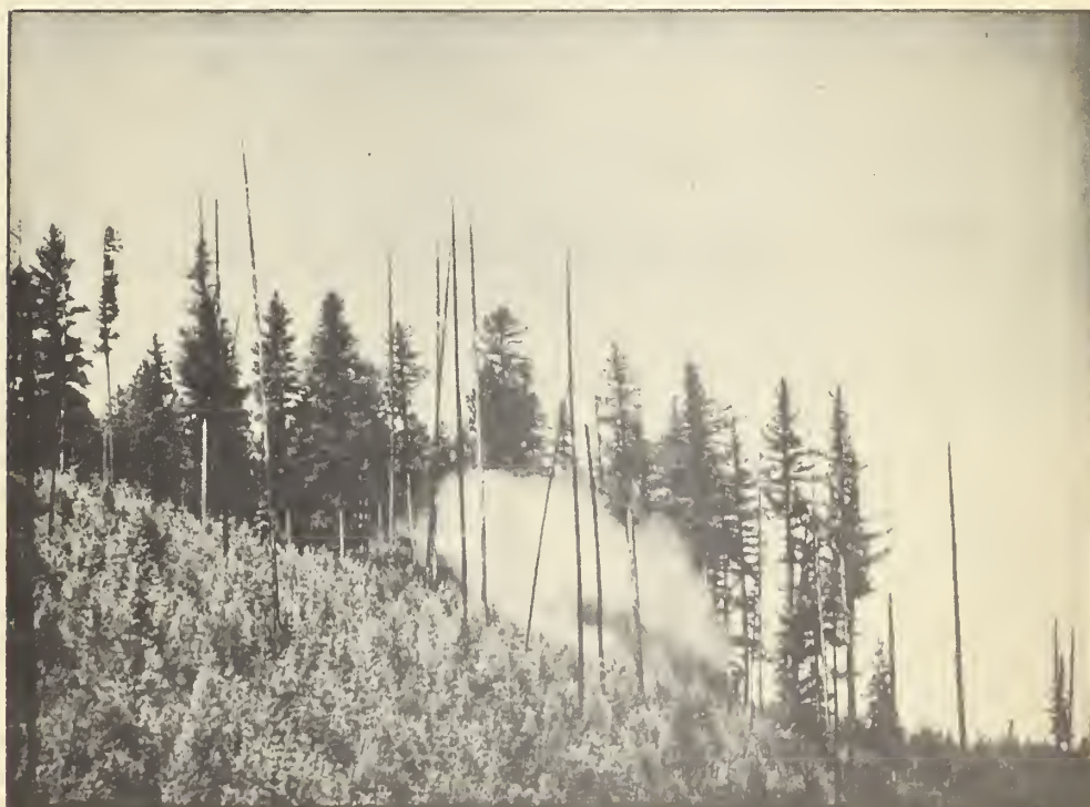
Figure B. The outrushing cascade of water from a bomb burst 50 feet above ground in a timber stand.
